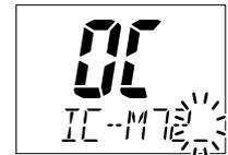
▨ The programmed opening comment is briefly displayed or scrolled when the transceiver is powered ON.
