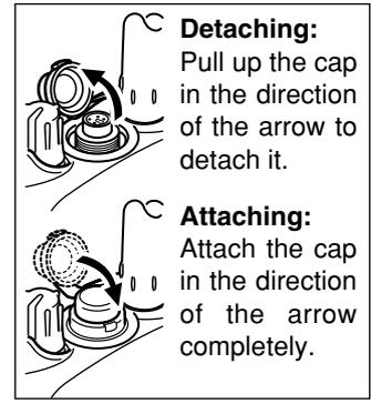
**IMPORTANT: KEEP** the transceiver's [SP MIC] connector cap attached when the speaker-microphone is not in use. Water will not get into the transceiver even if the cover is not attached; however, the terminals (pins) will become rusty, or the transceiver will function abnormally if the connector has become wet.
