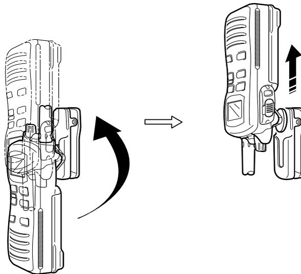
**⚠ CAUTION!:** HOLD THE TRANSCEIVER TIGHTLY WHEN HANGING OR DETACHING THE TRANSCEIVER FROM THE BELT CLIP.
