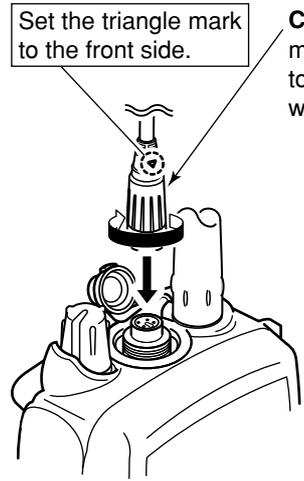
**CAUTION:** Attach the speaker-microphone's connector securely to prevent accidental dropping, or water intrusion in the connector.
