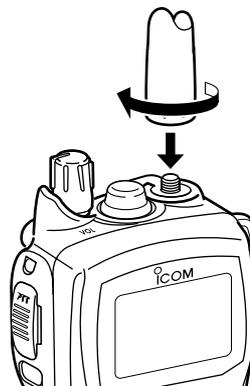
**CAUTION:** Transmitting without an antenna may damage the transceiver.
