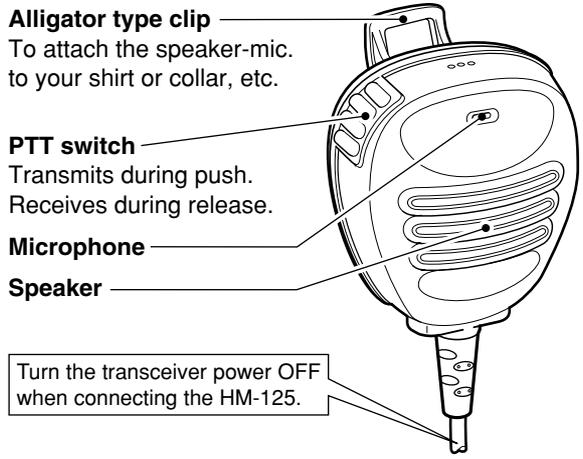
**NEVER** immerse the connector in water. If the connector becomes wet, be sure to dry it **BEFORE** attaching it to the transceiver.
